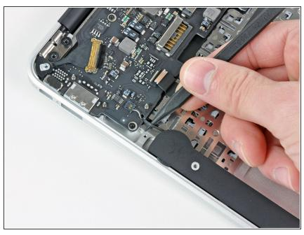
Use the tip of a spudger to de-route the right speaker cable from the slot cut into the logic board.
