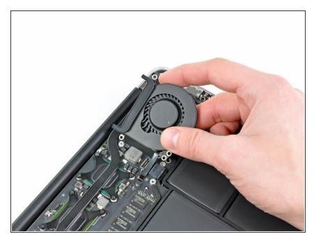
Lift the fan out of the upper case and carefully pull the fan ribbon cable out of its socket as you remove it from the Air.
