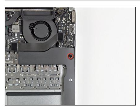
Remove the single 2.7 mm T5 Torx screw securing the left speaker to the upper case.
