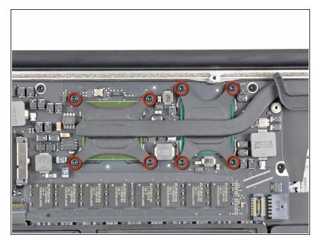
Remove the eight 2.5 mm T5 Torx screws securing the heat sink to the logic board.
