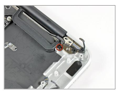
Push the antenna cable retainer out of the way and remove the 3 mm T5 Torx screw securing the end of the heat sink to the upper case.
