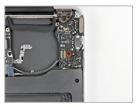
Remove the single 3.6 mm T5 Torx screw securing the I/O board to the upper case.
