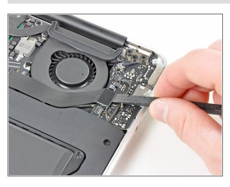
Use the flat end of a spudger to pry the I/O board cable connector upward out of its socket on the I/O board.
