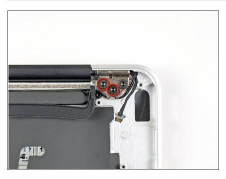
Remove the two 4.9 mm T8 Torx screw securing the antenna cable retainer on the left display hinge to the upper case.
