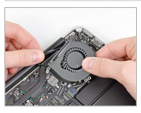
Lift the fan out of the upper case and carefully pull the fan ribbon cable out of its socket as you remove it from the Air.
