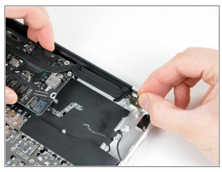
i Hold the antenna cables out of the way as you lift the heat sink end of the logic board out of the upper case.
