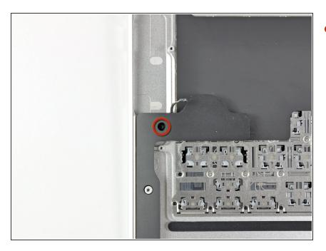
Remove the single 2.7 mm T5 Torx screw securing the right speaker to the upper case.
