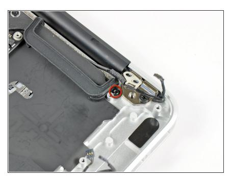
Push the antenna cable retainer away slightly and remove the 3 mm T5 Torx screw securing the end of the heat sink to the upper case.
