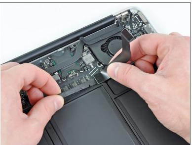
The following connector has an especially deep socket. Use care when disconnecting it.
