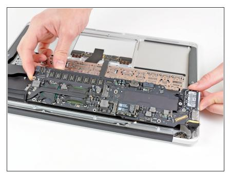
Carefully remove the logic board assembly from the upper case, minding any cables that may get caught.
