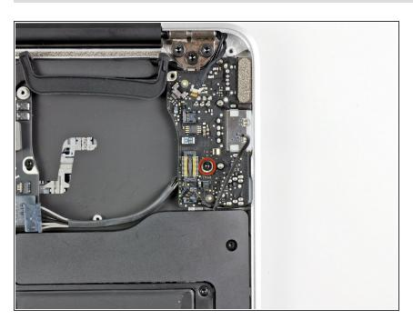
Remove the single 3.6 mm T5 Torx screw securing the I/O board to the upper case.
