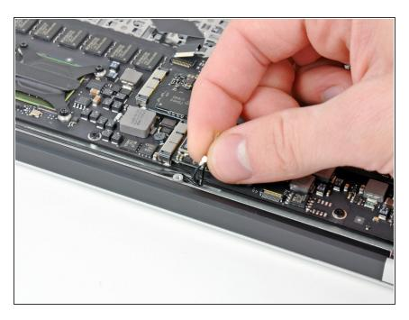
Gently de-route the antenna cables from the slot cut into the logic board.
