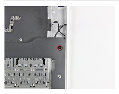
Remove the single 2.7 mm T5 Torx screw securing the left speaker to the upper case.
