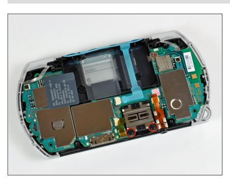
Remove both headphone jack and analog joystick screws using your #00 Phillips screwdriver.
