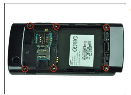
Remove the six 4.5mm #000 Phillips screws.
