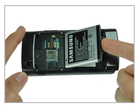
Place your finger on the bottom of the battery and lift to remove.
