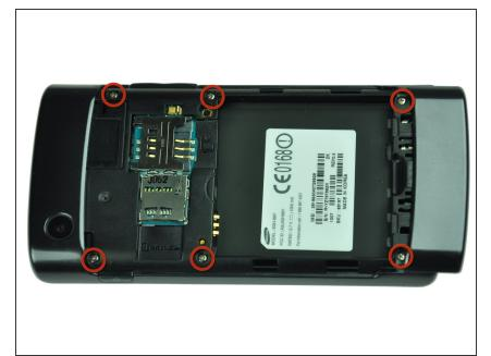
Remove the six 4.5mm #000 Phillips screws.
