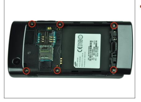
Remove the six 4.5mm #000 Phillips screws.
