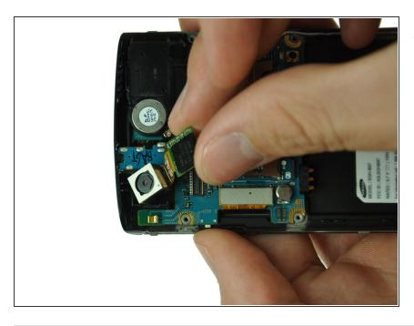
• Gently lift the camera assembly out of the plastic housing.
