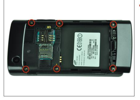
Remove the six 4.5mm #000 Phillips screws.
