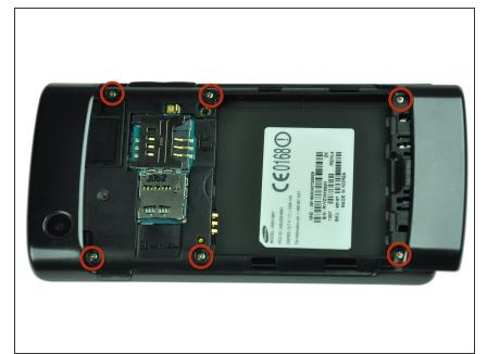
Remove the six 4.5mm #000 Phillips screws.
