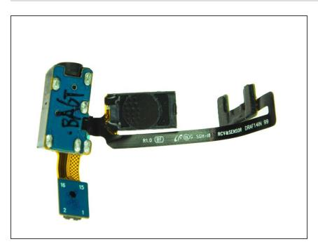
The earpiece is attached to the 3.5mm audio jack. You will need to replace the entire assembly. To reassemble your device, follow these instructions in reverse order.
