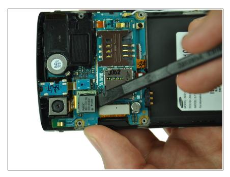
Use the spudger tool to pry up the chip labeled "NEC." This releases the chip.
