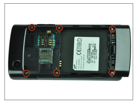
Remove the six 4.5mm #000 Phillips screws.
