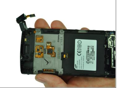
Gently pull up on the audio jack, taking the attached ribbon cable with it.
