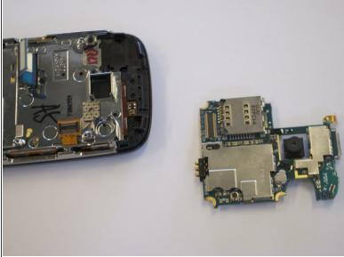
The circuit board will still be held on by a blue and black ribbon that is removed by gently pulling it upwards.
