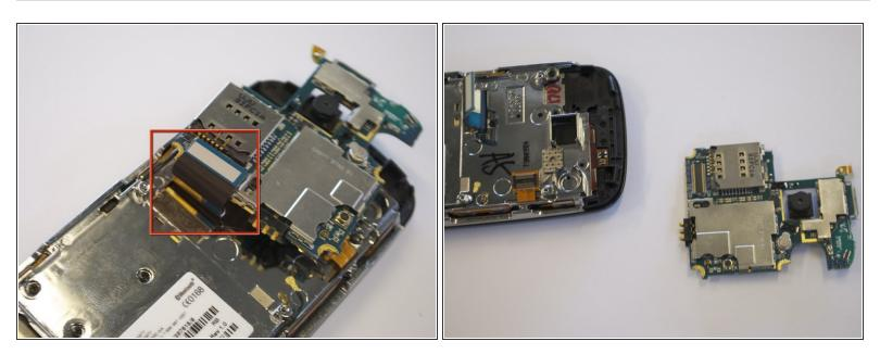
The circuit board will still be held on by a blue and black ribbon that is removed by gently pulling it upwards.
