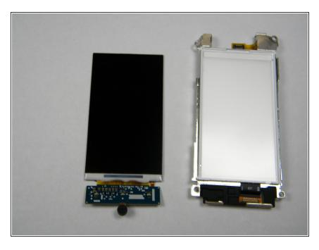
After lifting out the LCD screen, the screen and its housing should be separated as shown.
