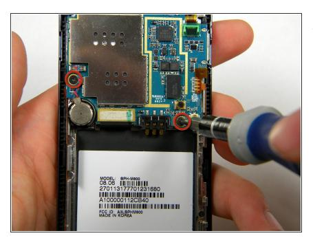
Remove the two 3.50mm screws connecting the motherboard to the case.
