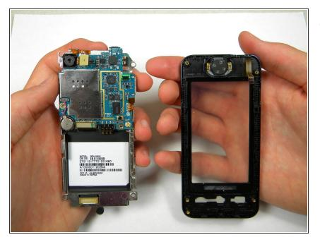
After removing lifting up on the motherboard, the front casing and center frame should be separated as shown.
