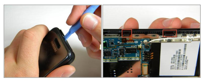
• Use the plastic opener tool to unhinge the locks around the edges of the phone.
