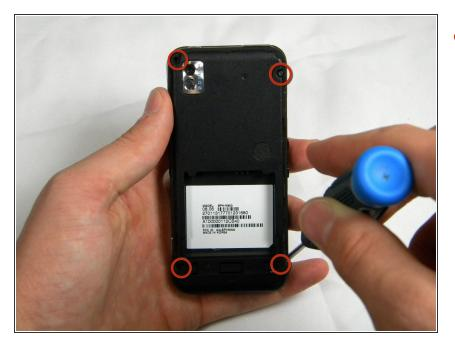
• Remove the four 4.45mm screws at the corners of the phone.
