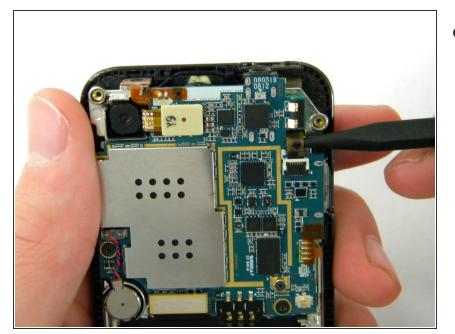
• Lift out the top right ribbon from its slot on the motherboard.
