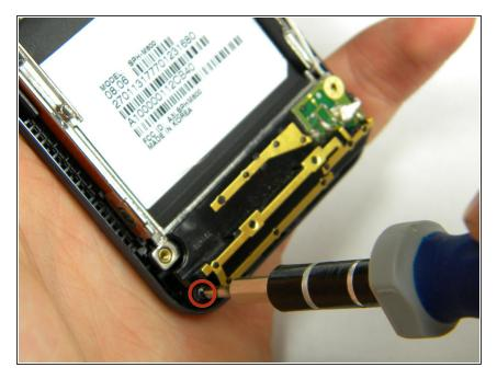
Using a phillips-head screwdriver, remove the 4.50mm screw holding the antenna in place.
