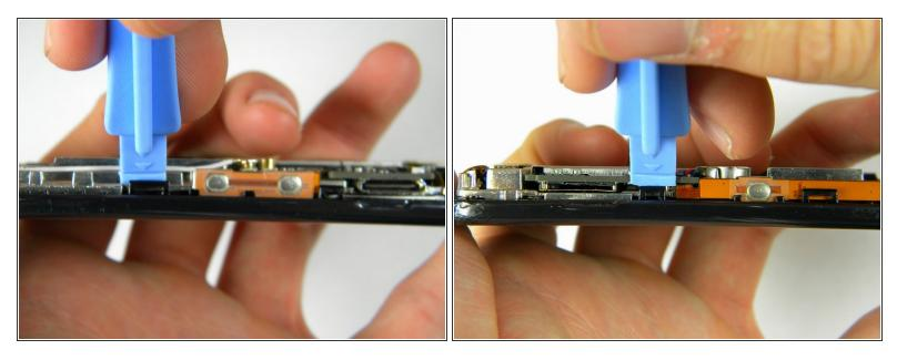
Use the plastic opener tool to unhinge the the locks on the side of the motherboard connecting it to the front casing.
