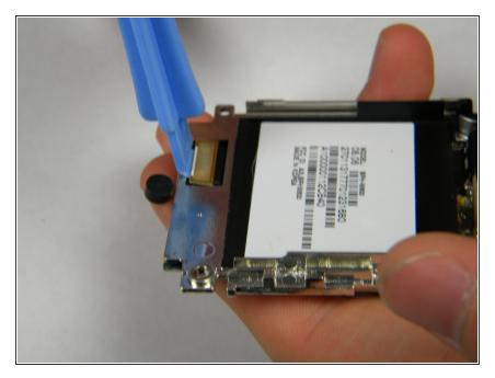
Using the plastic opener tool, detach the ribbon located on the bottom of the phone below the battery compartment.
