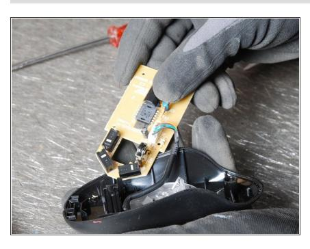
Remove the printed wiring board and store it separately.
