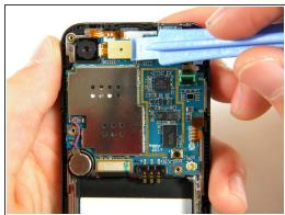
• Use the plastic opener tool to detach the three ribbons on the motherboard.
