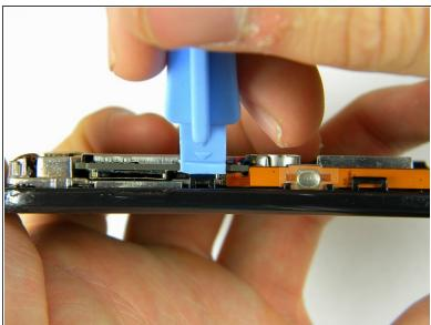
• Use the plastic opener tool to unhinge the the locks on the side of the motherboard connecting it to the front casing.
