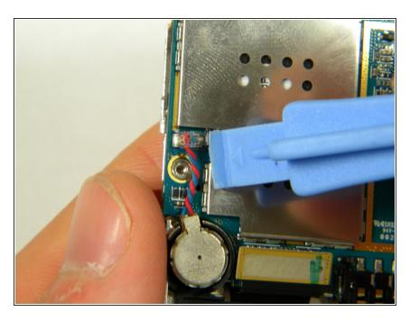
Using the plastic opener tool, pry the speaker connector away from the back of the motherboard.
