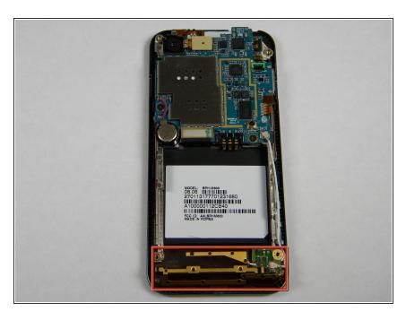
With the screws removed, locate the antenna.
