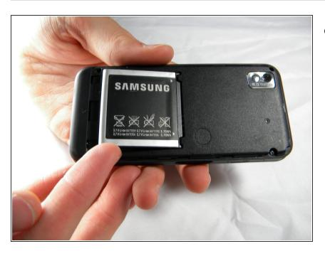
Hold the phone firmly in one hand and lift the battery up by using the notches to grip the battery.
