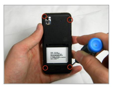
Remove the four 4.45mm screws at the corners of the phone.
