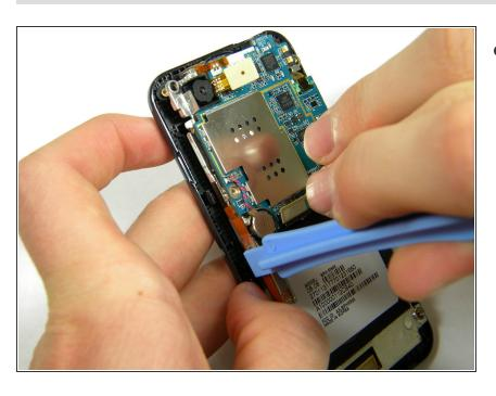
Lift the motherboard away from the front casing.
