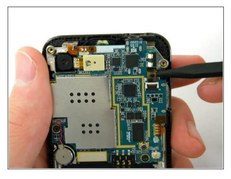
Lift out the top right ribbon from its slot on the motherboard.
