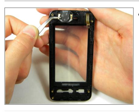
Using tweezers to grasp the pins of the speaker, gently lift the speaker up out of its setting in the front case.
