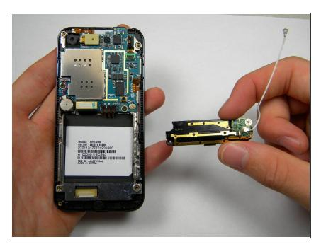
Gently lift up on the antenna and remove it from the back of the device.
