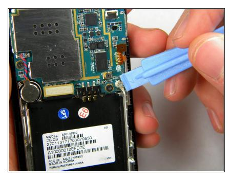
Using the plastic opener tool, squeeze gently on the antenna cable connector and lift to remove the connector from its position.
