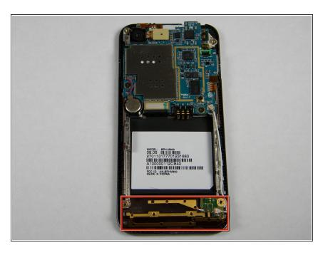
With the screws removed, locate the antenna.
