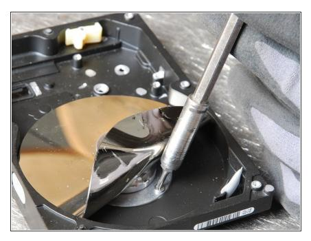
Unscrew the bottom circular plate with the motor.
