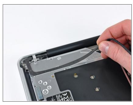
Peel the camera cable off the adhesive securing it to the optical drive.
