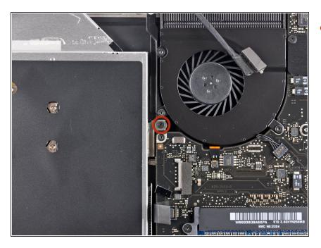
Remove the single 3.5 mm Phillips screw securing the inner side of the optical drive to the upper case.
