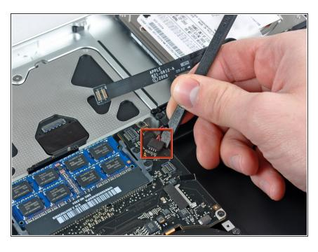
Using the flat end of a spudger, pry the subwoofer/right speaker connector straight up off the logic board.
