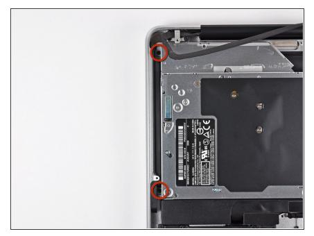
Remove the two 3.5 mm Phillips screws securing the outer side of the optical drive to the upper case.
