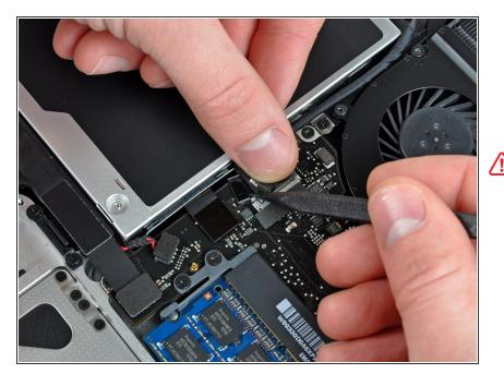
Apple sticks a small strip of clear plastic with adhesive applied to one side to the logic board behind the camera cable connector to keep it in its socket. When moving it out of the way, be sure not to break any surface-mount components off the logic board.
