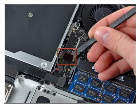
• Use a spudger to pry the optical drive connector straight up off the logic board.
