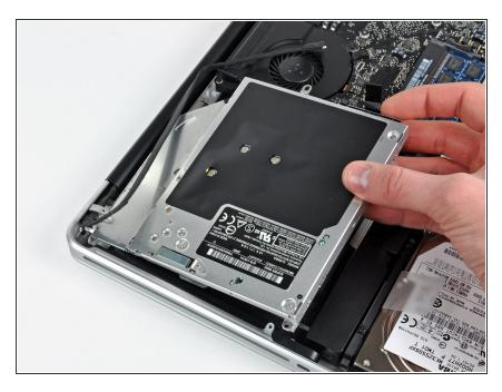
• Lift the optical drive from its left edge and pull it out of the upper case.
