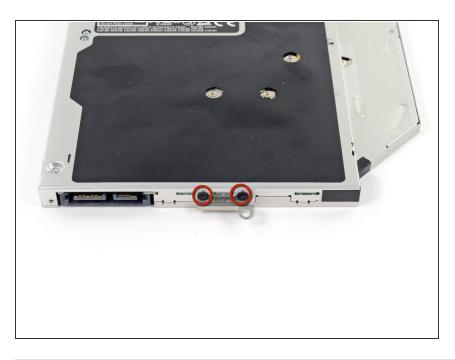
Remove the two black Phillips #0 screws securing the small metal mounting bracket. Transfer this bracket to your new optical drive or .
