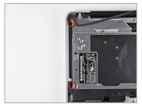
Remove the two 3.5 mm Phillips screws securing the outer side of the optical drive to the upper case.
