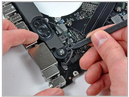
(i) If your microphone is still inserted into its void in the left speaker housing, use the tip of a spudger to lift it out.
