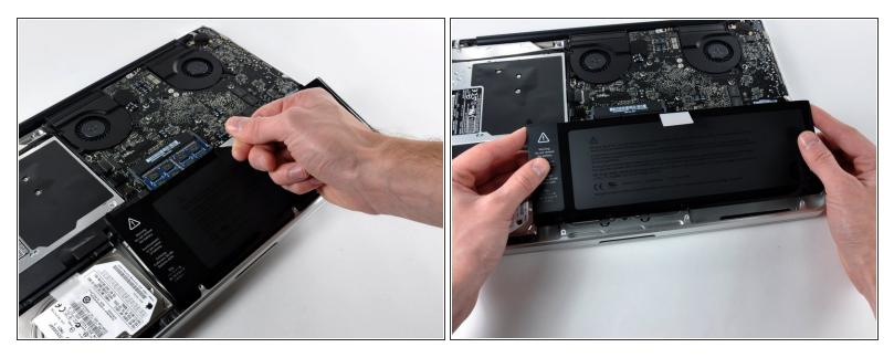
• Lift the battery by its plastic pull tab and slide it away from the long edge of the upper case.
