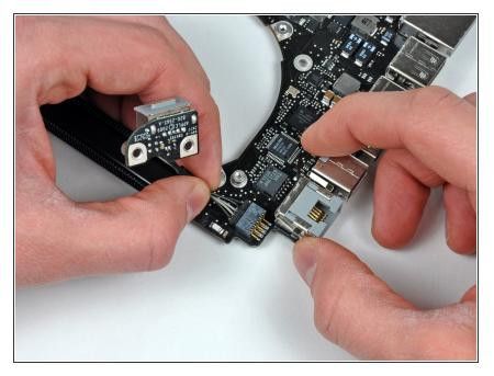
Disconnect the DC-In Board connector from the logic board by pulling it straight away from its socket.
