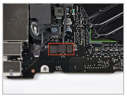
• Remove the small strip of tape covering the left speaker connector.
