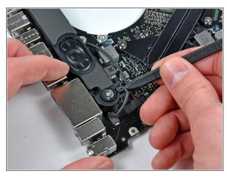
into its void in the left speaker housing, use the tip of a spudger to lift it out.
