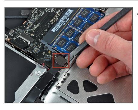
Use the flat end of a spudger to pry the hard drive/IR sensor cable connector up off the logic board.
