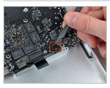
Use a spudger to pry the battery indicator ribbon cable connector up off the logic board.
