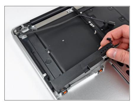
Lift the subwoofer and right speaker assembly out of the upper case.
