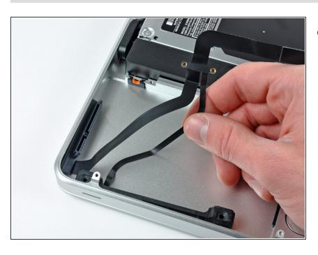
Carefully peel the IR sensor/sleep light ribbon cable off the adhesive securing it to the upper case.
