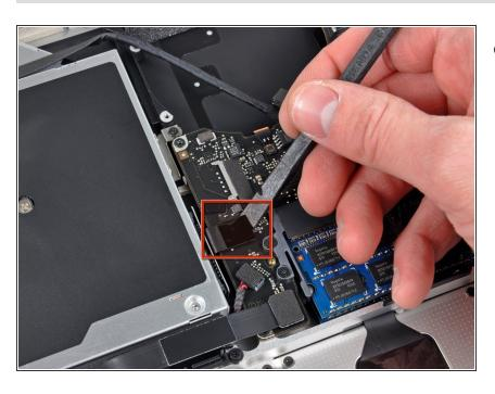
Use the flat end of a spudger to pry the optical drive cable connector up off the logic board.
