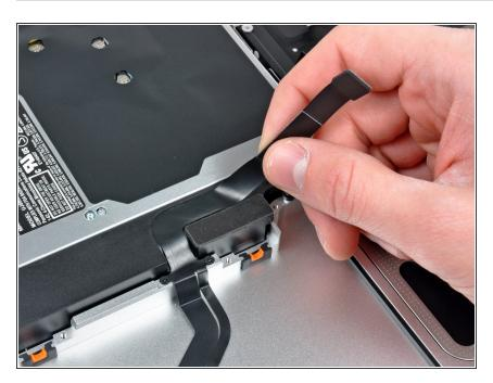
Carefully peel the hard drive cable off the adhesive securing it to the right speaker housing.
