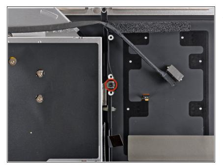
Remove the single 3.5 mm Phillips screw securing the inner side of the optical drive to the upper case.
