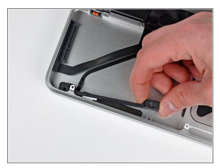
Slide the hard drive and IR sensor bracket away from the edge of the upper case.
