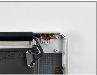
Remove the outer two T6 Torx screws securing both display hinges to the upper case (four screws total).
