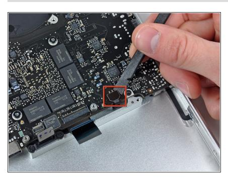
Use a spudger to pry the battery indicator ribbon cable connector up off the logic board.
