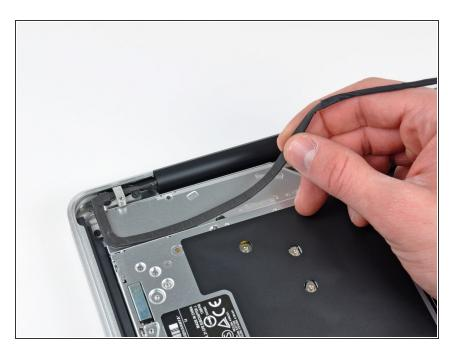
Peel the camera cable off the adhesive securing it to the body of the optical drive.
