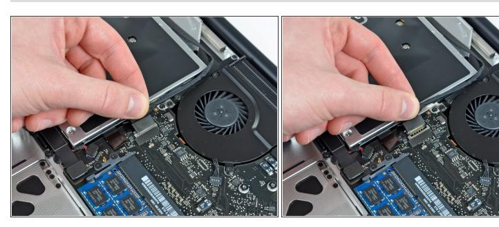
Pull the camera cable away from its socket on the logic board.
