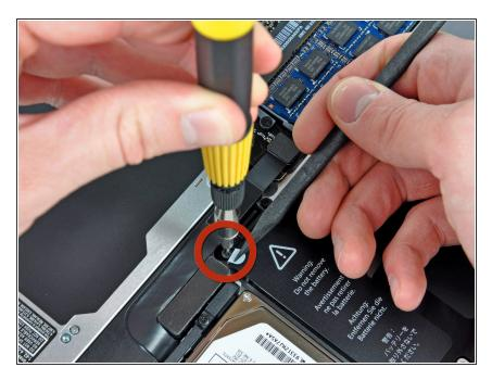
Use the tip of a spudger to bend back the finger of the "Warning: Do not remove the battery" sticker while you remove third five-point Pentalobe screw hidden underneath.
