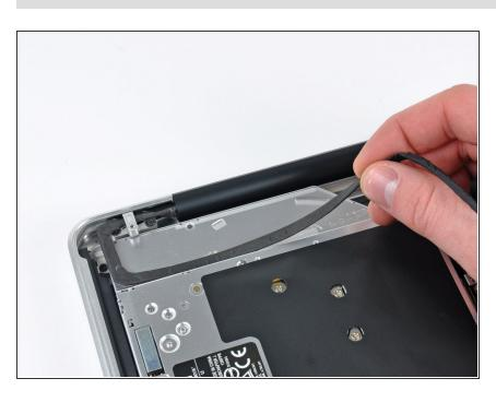
Peel the camera cable off the adhesive securing it to the body of the optical drive.
