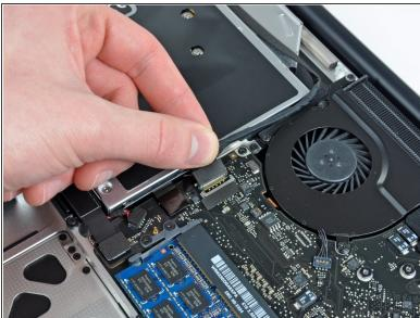
Pull the camera cable away from its socket on the logic board.
