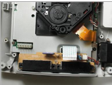
Remove the four 14mm Philips #02 located on the controller board.
