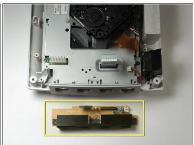
Remove the controller board by lifting it up from the controller port.
