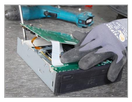
Unscrew and remove the PWB.
