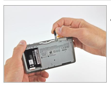
Remove the stylus from the lower case.
