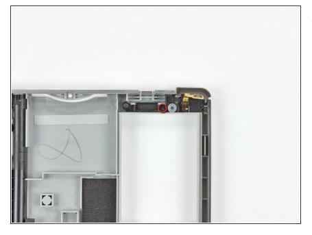
• Remove the 3.6 mm Phillips screw from the right shoulder button cover.
