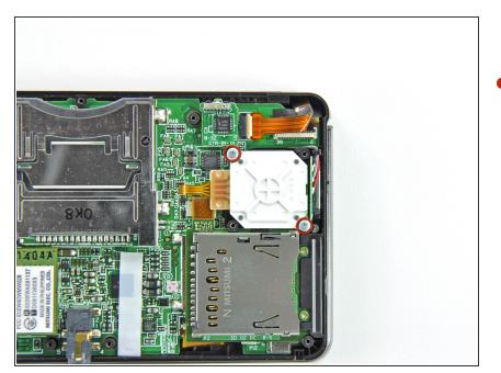
Remove the two 7.7 mm Phillips screws securing the back of the Circle Pad to the motherboard.
