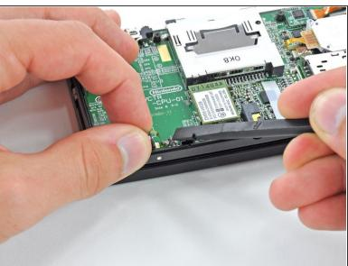
Use the flat end of a spudger or your fingernail to flip up the retaining flap on the Microphone ribbon cable ZIF socket.
