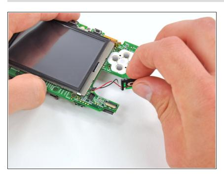
Remove the volume switch from the motherboard.
