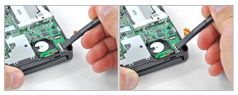
Use the flat end of a spudger or your fingernail to flip up the retaining flap on the camera ribbon cable ZIF socket.
