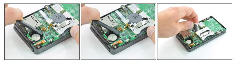
• Use the flat end of a spudger or your fingernail to flip up the retaining flap on the Circle Pad ribbon cable ZIF socket.
