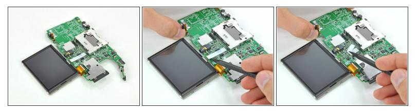
(i) Set the motherboard assembly down so that the lower LCD is side-by-side with the motherboard.
