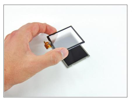
Gently lift the touchscreen up to completely separate it from the lower LCD.
