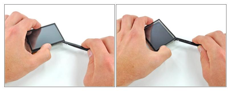
Repeat the above procedure for the remaining two corners to pry the touchscreen off the LCD frame.
