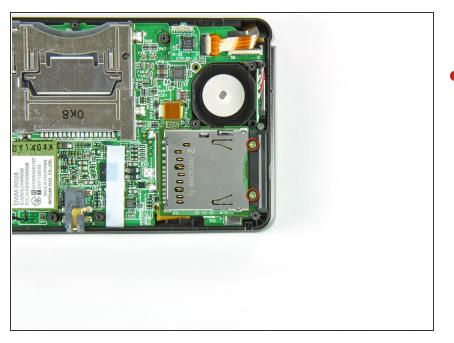
Remove the two 4.5 mm Phillips screws securing the SD board to the motherboard.
