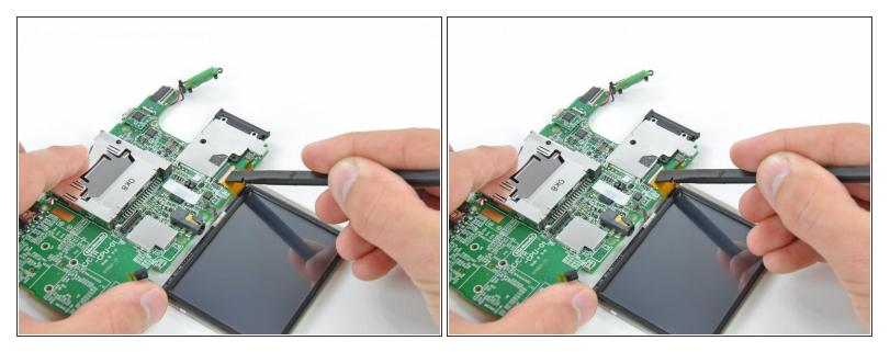
Use the flat end of a spudger or your fingernail to flip up the retaining flap on the lower LCD data ribbon cable ZIF socket.
