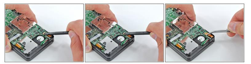
• Use the flat end of a spudger or your fingernail to flip up the retaining flap on the speaker assembly ribbon cable ZIF socket.
