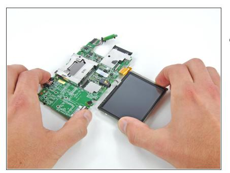
Grasp the lower display assembly and pull it directly away from the motherboard.
