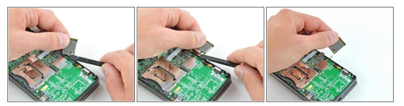
(i) Lift the Wi-Fi board off the motherboard and rotate it so that the bottom side is facing up.
