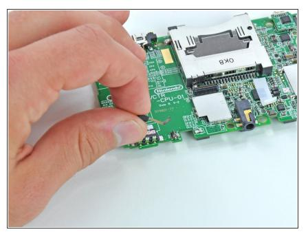
• Lift the microphone and its attached ribbon cable off the motherboard.
