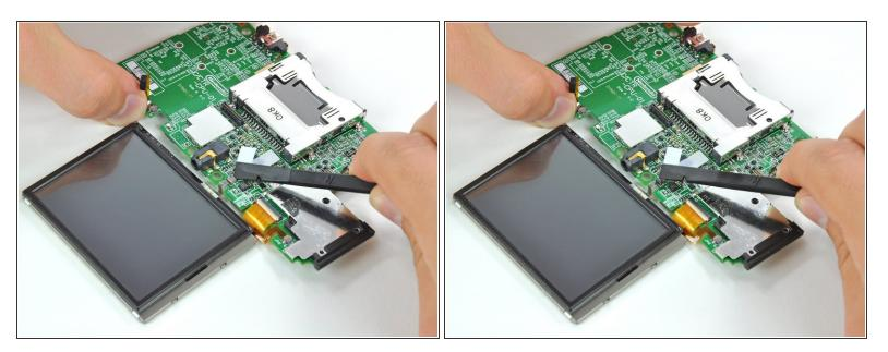
Use the flat end of a spudger or your fingernail to flip up the retaining flap on the touchscreen ribbon cable ZIF socket.
