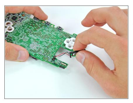
• Remove the volume switch from the motherboard.
