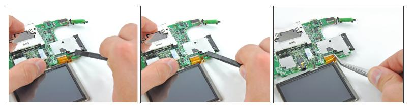
• Use the flat end of a spudger or your fingernail to flip up the retaining flap on the lower LCD power ribbon cable ZIF socket.
