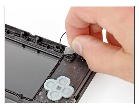
• Peel the silicone cover from the back of the power button.
