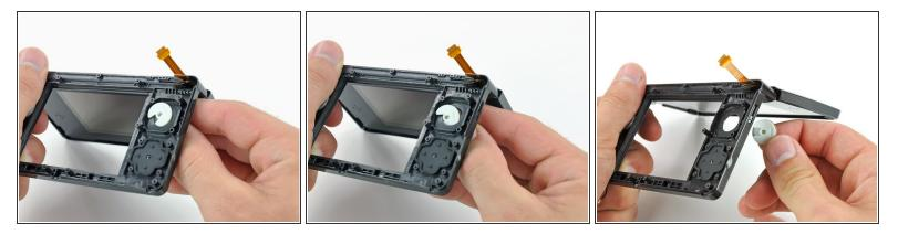
(i) Open the 3DS and hold it so that the bottom of the buttons are facing upward.
