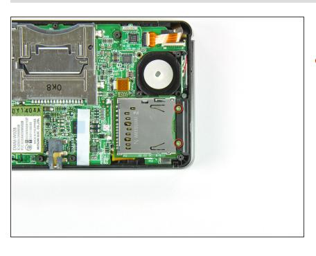
Remove the two 4.5 mm Phillips screws securing the SD board to the motherboard.
