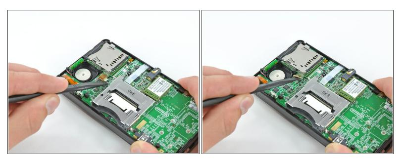
Use the flat end of a spudger to pry the SD board ribbon cable connector off its socket on the motherboard.
