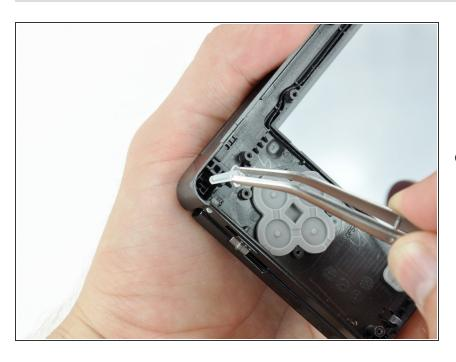
Before continuing with disassembly, use a pair of tweezers to remove the clear plastic diffuser for the wireless notification LED. The small piece is likely to fall out on its own, and may be difficult to find if it lands on the floor.
