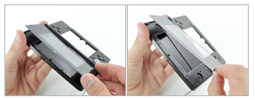
With all of the sides free, lift the upper display front panel off the display bezel.
