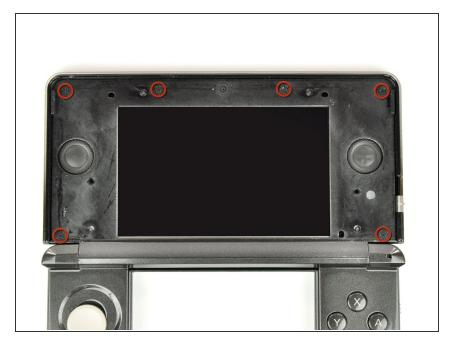
Remove the six 3.6 mm Phillips screws securing the rear display bezel to the front display bezel.
