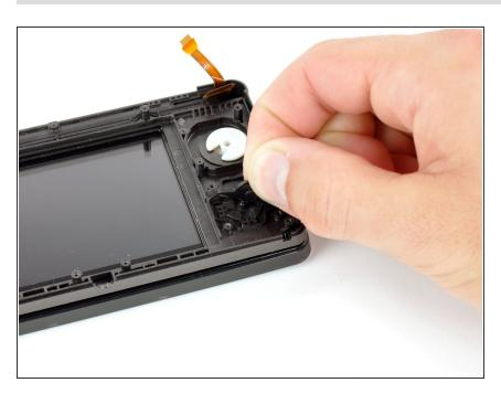
Peel the black silicone cover off the back of the D-pad.
