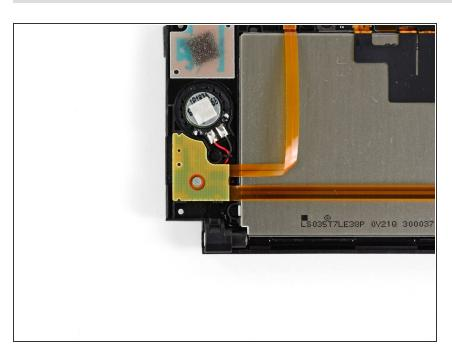
Remove the 2.5 mm Phillips screw securing the right speaker board to the upper display bezel.
