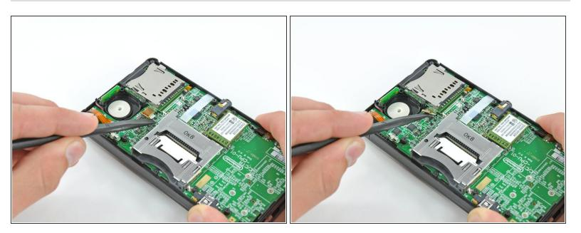
Use the flat end of a spudger to pry the SD board ribbon cable connector off its socket on the motherboard.
