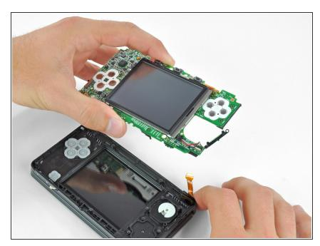
Remove the motherboard assembly from the rest of the device.
