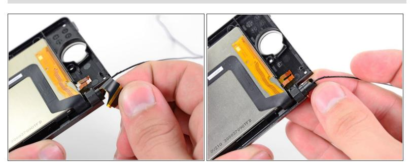
Gently roll the upper LCD ribbon cable and camera ribbon cable together and insert them into the hinge opening.
