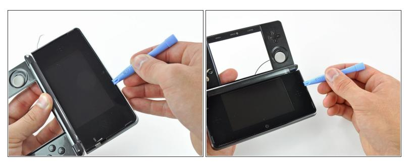
Continue prying the remaining sides of the front panel by sliding the plastic opening tool down each edge.
