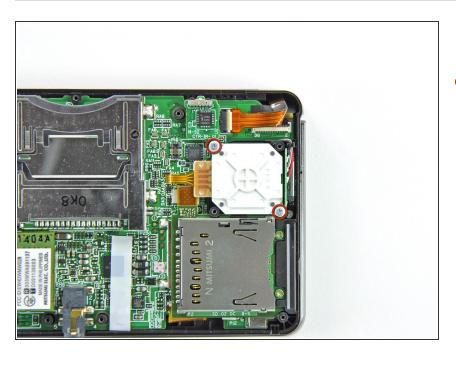
Remove the two 7.7 mm Phillips screws securing the back of the Circle Pad to the motherboard.
