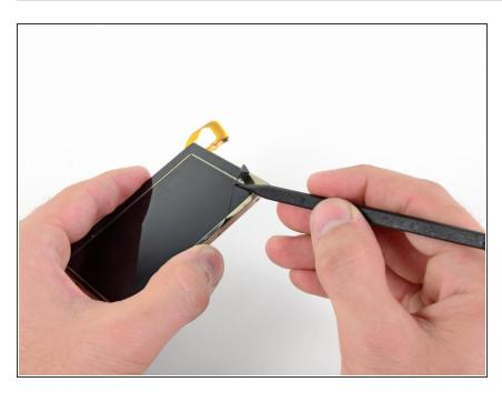
A strip of black adhesive tape holds the upper LCD to the display bezel.
