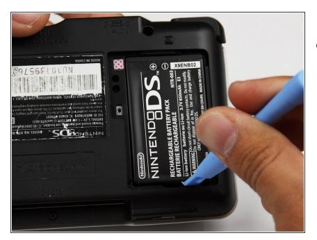
Use a plastic opening tool or spudger to pry out the battery from the bottom. If a plastic open tool or spudger isn't available, your fingernails may work.
