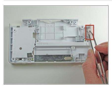
Use a pair of tweezers to carefully remove the power switch.
