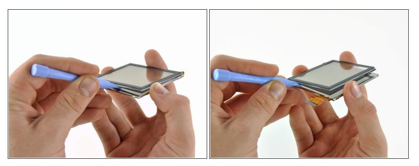
Continue sliding the plastic opening tool along the bottom and up the left edges of the LCD to separate the touchscreen from the LCD.
