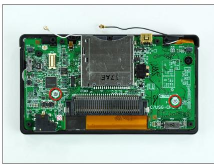
Remove the two 3.4 mm Phillips screws securing the motherboard to the upper case.
