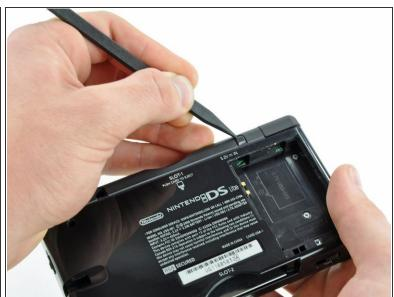
Use the tip of a spudger to pry both rubber feet off the DS Lite.
