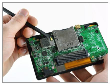
Use the flat edge of a spudger to pry the Wi-Fi antenna connector straight up from its socket on the Wi-Fi board.
