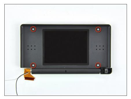
Remove the four 3.4 mm Phillips screws securing the rear display bezel to the front display bezel
