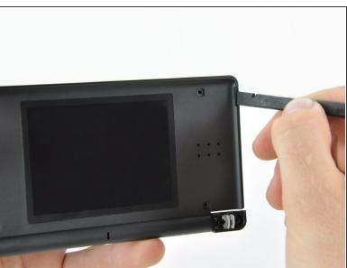
Use the edge of a spudger to pry both rubber pads out of the front display bezel.
