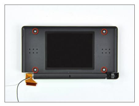
Remove the four 3.4 mm Phillips screws securing the rear display bezel to the front display bezel
